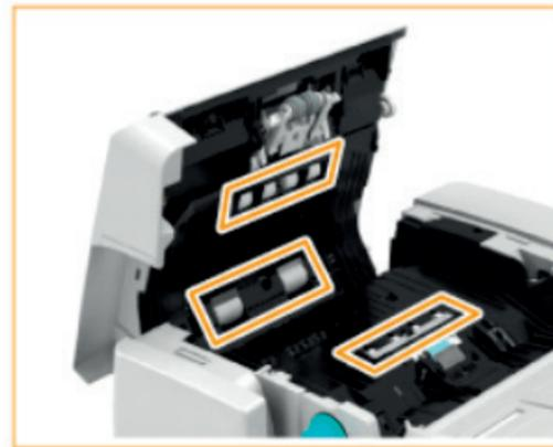
**2b** Make sure that no bits of paper gets into the groove of the multiple sheet feed detection sensor. If this happens, remove using a soft cloth.
