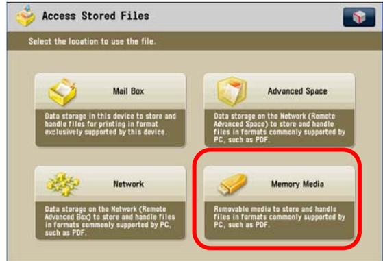
3. Insert the USB Memory stick into the USB Connection on the right hand side of the panel. Touch the Memory Media on the screen.
